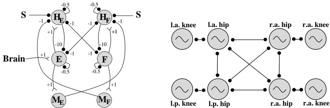
Figure 1: **Left:** Connectivity within one oscillator.  $B$  is the tonic input,  $M_E$  and  $M_F$  are the motoneurons for the extensor and flexor muscles resp., and  $E, F, H_E$  and  $H - F$  are interneurons. The input connection from the brainstem is also shown. **Right:** Coupling among the hip and knee oscillators.
