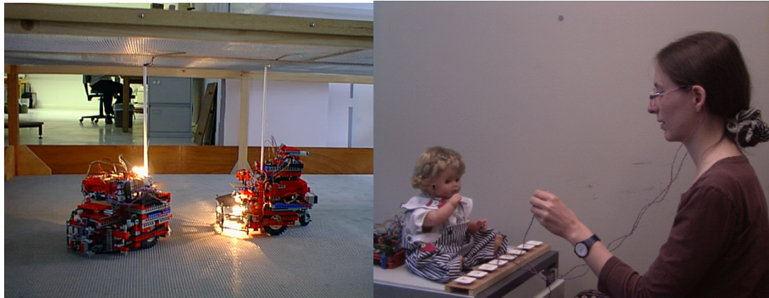
Figure 2: The experiments are based on an imitative scenario, namely following behavior (left) and mirroring of arm and head movements (right), whereby the learner robot replicates the movements of the teacher.
