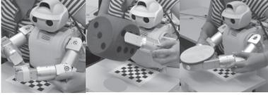
Figure 2: Set-ups of 3 experiments. *Tea task*: put the piece of sugar into the cup. *Cube task*: grasp the cube, lift it, and put it on top of the pedestal. *Tray task*: grasp the tray with two arms, lift it, and move it forward.
