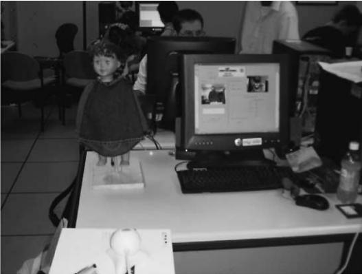
Fig. 3. The setup for Robota learns to dress up. Project by Alex Chan, Johnny Li and Siu Lun Wu. The camera is placed in front of Robota at a fixed distance of 60 cm. The camera output is visible on the PC screen.
