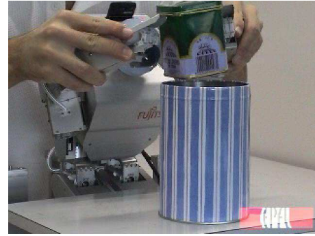
Fig. 2. A demonstrator is teaching a movement which requires bending of the torso to the humanoid robot HOAP-2
