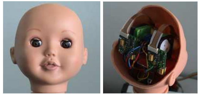
Fig. 6. 3 degrees of freedom pair of eyes for Robota. To ensure that the overall aesthetic of the robot is conserved, we made sure that only visible part of the mechanism would be the eyes.
