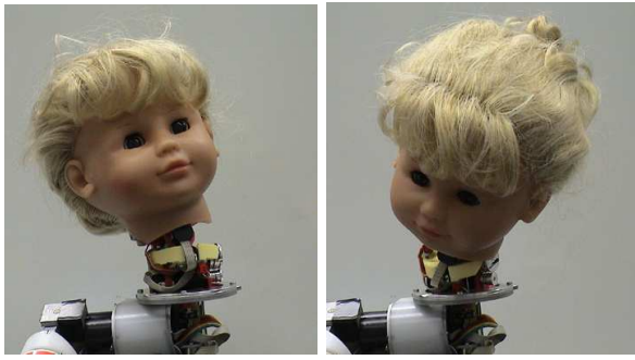
Fig. 8. Realization of the three degrees of freedom neck.
