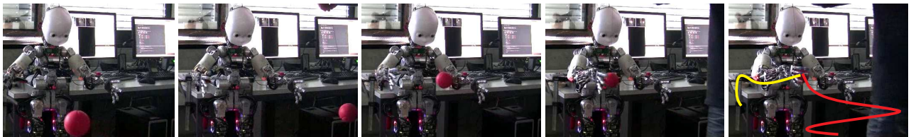
(b) A ball is connected to a human hand with a thin wire; A human generate a ball trajectory by hand in the experiment.
