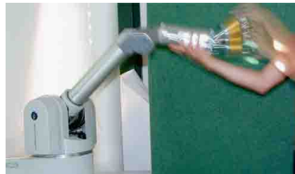
Fig. 1. The figure shows a human teacher physically interacting with the robot to make it less stiff. This is done by perturbing it around the current equilibrium point.
