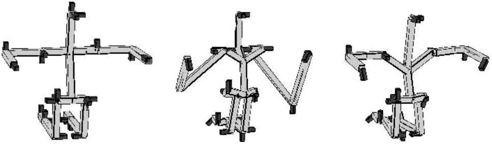
Fig. 11. Left: The Hoap3 “real” body schema, when standing on its knees. Middle: The objective body schema that was learned by the system when looking only at its hands and feet. It is not exactly the same, but the sensory relationships of both schemas (i.e. the subjective body schemas) are the same, when considering only vision of the hands and feet. Right: The body schema learned when also looking at elbows, knees, shoulders and the waist. The darker sticks indicate the rotation axis of each joint. There are three DOFs at the shoulders and the hips.
