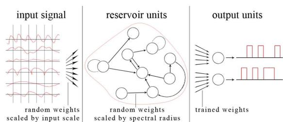
The input gait motion data is normalized and re-scaled and then fed to the reservoir neurons.
