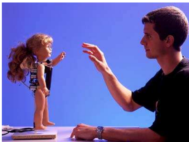
Figure 1: A PocketPC mounted with a FlyCam Camera tracks the motion of the user and sends commands to the microcontrollers and servos of Robota, so that it can imitate the motion of the head and arms of a user.
