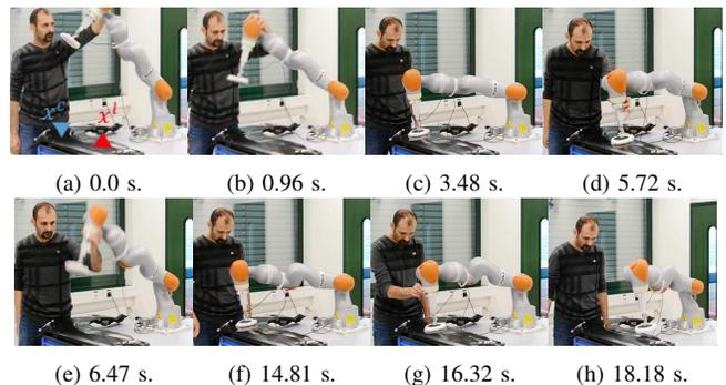
Fig. 6: Snapshots of the motion of the robot while performing Scenario 1 under perturbations. As  $\eta = 15$  and  $\rho = 20$ , the effective transition region is 5cm. Due to the closed loop implementation of (1), the robot complies with the human operator in all directions.
