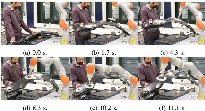
Fig. 5: Snapshots of the motion of the robot in a dynamically changing environment. (a) is the initial location. In (c), the robot makes contact with the surface at  $x^c$ . In (d), the robots slides on the surface while the surface's orientation is changed. In (e), the robot reaches  $x^l$  and, consequently, leaves the surface as depicted in (f).
