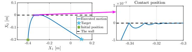
(b) The modulation function is disabled by setting  $M = I$ . As the force of impact is nonzero, ( $\approx -19.4N$ ), not only is the contact unstable causing the robot to bounce on the surface, but also the robot does not contact the surface at the desired location.
