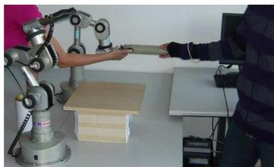
Fig. 1. In a scenario used for collecting data and preliminary experiments, a robotic arm (KATANA from Neuronics) assists a human collaborator to transport an object. The human wears a motion suit that captures motion of her joints, thus a robot knows the posture of the human arm at each time step. Another person kinesthetically guides the robot demonstrating its part of the task.
