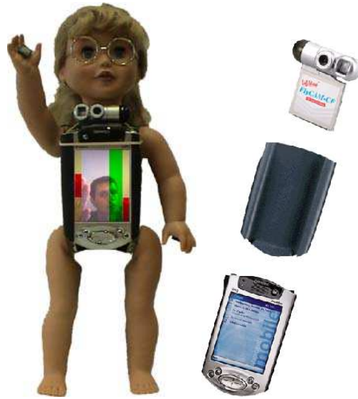
Fig. 1. Robota , and the connection of a small camera to the iPAQ PocketPC , using an Expansion Pack to read Compact-Flash memory cards.
