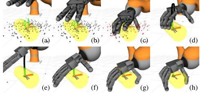
Fig. 6: **Exp 1**: Images of the exploration and grasping procedure with the cylinder. On frame (d), the hand automatically switches to a grasping motion, and moves up to approach the object from above, until grasping on frame (h). The reference frames made out of three RGB segments represent the real object's position and the estimated one. The estimated object's pose can be seen moving towards the real one as the PF converges using tactile information
