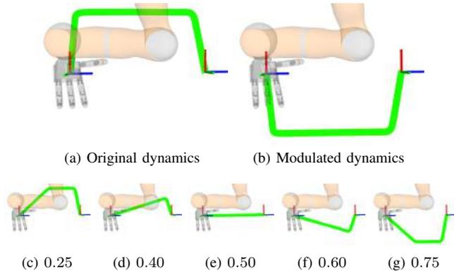
Fig. 13: **Exp 2b**: The RGB frames on the left and right correspond respectively to the starting point and the target. Seen from above, in green, trajectories of the DS. **Top**: The original and modulated dynamics. **Bottom**: The resulting dynamics with different levels of activation  $h_s$ . With  $h_s = 0.50$ , the dynamics reach in a straight line.
