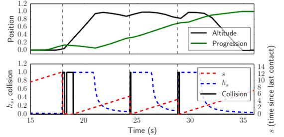
Fig. 12: **Exp 2a simulation**. **Top**: Evolution of the altitude of the hand (normalized) and the progression of the task (horizontal position between start and end points, normalized between 0 and 1). **Bottom**: Evolution of the external signal  $s$  (time since last collision), activation function  $h_s(s)$ , and the collision status. The vertical dotted lines correspond to collisions with obstacles, see fig. 11.
