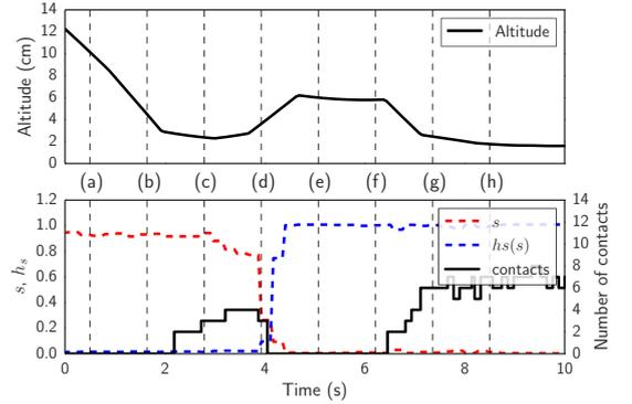
Fig. 7: **Exp 1**: Evolution of the external signal  $s$ , activation function  $h_s(s)$  and the altitude of the hand during one exploration trial. The labels (a)-(h) correspond to the steps of exploration in fig. 6.
