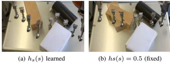
Fig. 16: **Exp 2b:** Evolution of the obstacle avoidance task with the controller activated (a) or not (b). The end-effector reaches from left to right. In both cases, the desired velocity is tracked using a passive DS controller.
