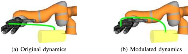
Fig. 2: **Exp 1:** In green, reaching trajectories for the original and modulated dynamics. The modulated dynamics force the trajectory to approach the object from above in order to avoid collisions with the fingers.
