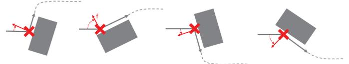
Fig. 14: **Exp 2b**: Schematic of the demonstrated trajectories. In red, the collision point and the force sensed during the collision. The end-effector follows the shape of the objects after contact, then continues again in a straight line after a few seconds.
