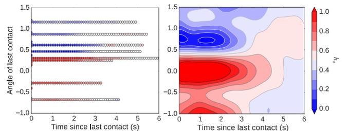
Fig. 15: **Exp 2b**. **Left**: Data from the demonstrations. Each horizontal line corresponds to one demonstration. **Right**: Learned function  $h_s(s)$ , using Gaussian Process Regression (GPR).
