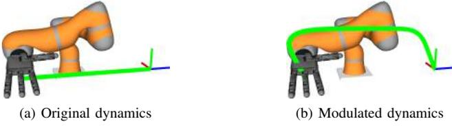
Fig. 8: **Exp 2a**: In green, reaching and avoiding trajectories corresponding to the original and modulated dynamics. The RGB frame on the right corresponds to the target. The modulated dynamics force the end-effector to go above obstacles and avoid collision with it.
