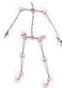
Figure 1: Positions of the motion-capture markers for gait analysis.
