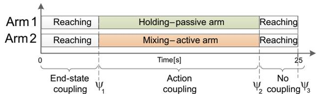
Figure 2: The identified motion segments for each arm, and corresponding coupling.
