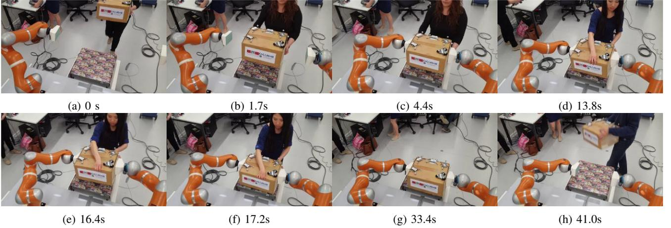
Fig. 4: Snapshots of the robots’ motion. In (a) and (b), the virtual object based motion generator guides the robots towards the moving object. In (c), the robots make secure contacts with the object. In (d), (e), (f), The robots remain in contact with the object even under external perturbations. In (g), the object is at a desired location, where a third operator hoists it as illustrated in (h). The corresponding video is available on-line: <https://youtu.be/MZikIS-rSn4>.
