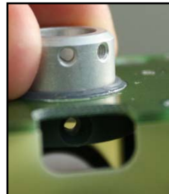
Figure 12: Insertion of the male connector
