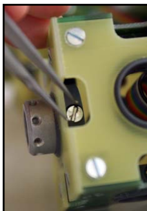
Figure 14: Fastening of the male connector with a screw
