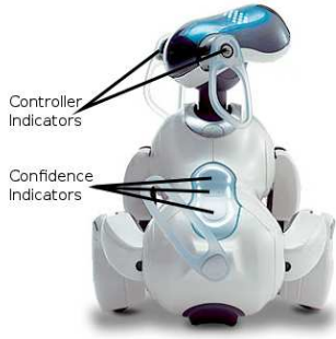
Fig. 2. The robot used in our experiments. Feedback to the user was given via LEDs on the robot’s surface. The robot’s ears change color based on which box’s output the arbitrator is currently running on the robot (red for teacher, blue for student, green for default). The robot’s back indicates the confidence value associated with the current output.
