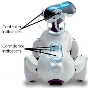
Fig. 2. Our robot. Feedback to the user was given via LEDs on the robot’s surface. The robot’s ears change color based on which output the arbitrator has selected (red for teacher, blue for student, green for default). The robot’s back indicates the confidence value associated with the current output.
